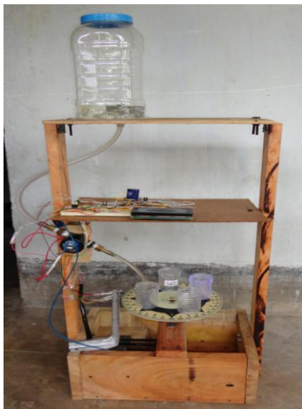
Fig.2: Whole setup of Liquid Filling Machine
